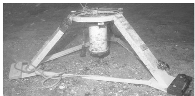
Fig. 3 Photograph of the mooring current system used in our observation system.
