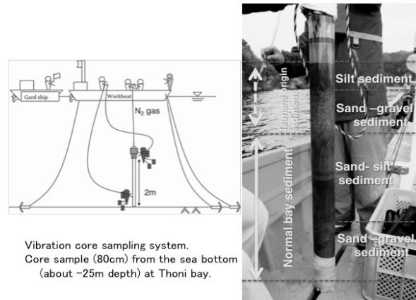
Fig.5 Vibration core sampling and core sample from Tohni Bay Seismic survey and the vibration core sampling were carried out to examine thickness of the outer layer sediment (Fig-5). It was revealed that tsunami
