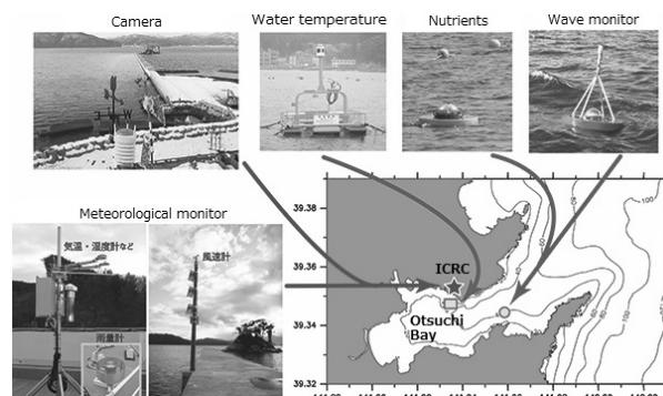
Fig. 1. Monitoring system in Otsuchi Bay
