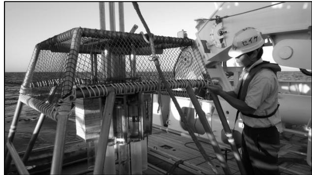
Fig. 2. Multiple sediment core sampler on the R/V Shinsei-maru.
