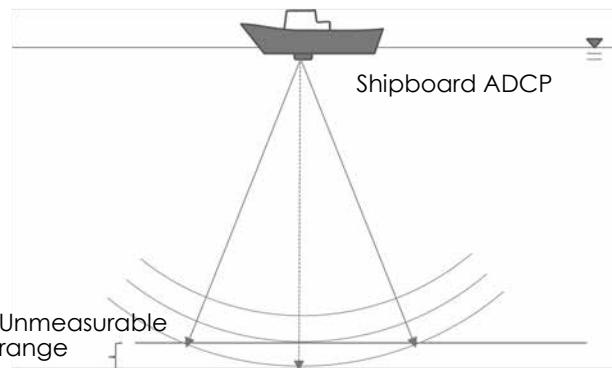
So, we lower the ADCP by using a towed fish in order to make it close to the seafloor and diminish the unmeasurable range.
