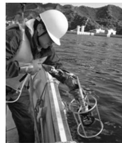
Fig. 4. Measurement of CTD profile.
