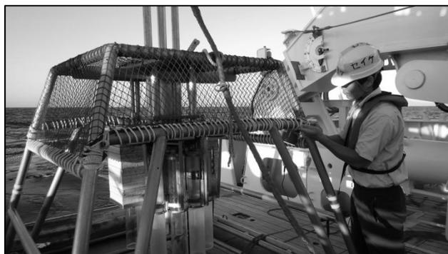
Fig. 2. Multiple sediment core sampler on the R/V Shinsei-maru.
